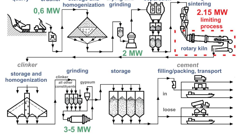
Fig. 2: Basic process chain in the cement industry (source: based on VDZ)
