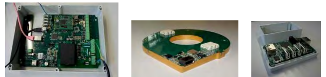
GridBox hardware, small form factor Rogovsky coil, data module
