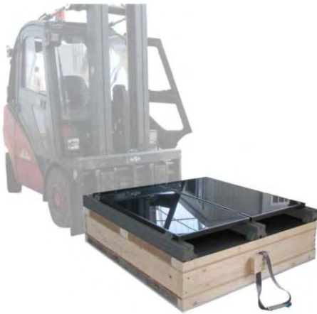
Abbildung 15: modular specimen of the prototype of wood prefabricated building component with PV [Building skin as electricity source: The prototype of a wooden BIPV facade component, 2011]
