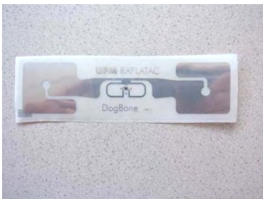
Abbildung 58: Transponder UPM Raflatac DogBone
