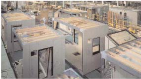
Computer-managed production lines realize efficient production of sophisticated, high quality houses.
